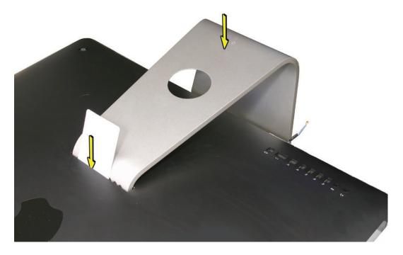
4. Insert the access card as far as it will go. Gently lift the stand approximately two inches to unlock the clutch mechanism, and then remove the access card. The clutch mechanism should now be unlocked.
